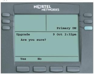
4. Press **Yes** to confirm the upgrade or press **No** to return to the Upgrade screen.
